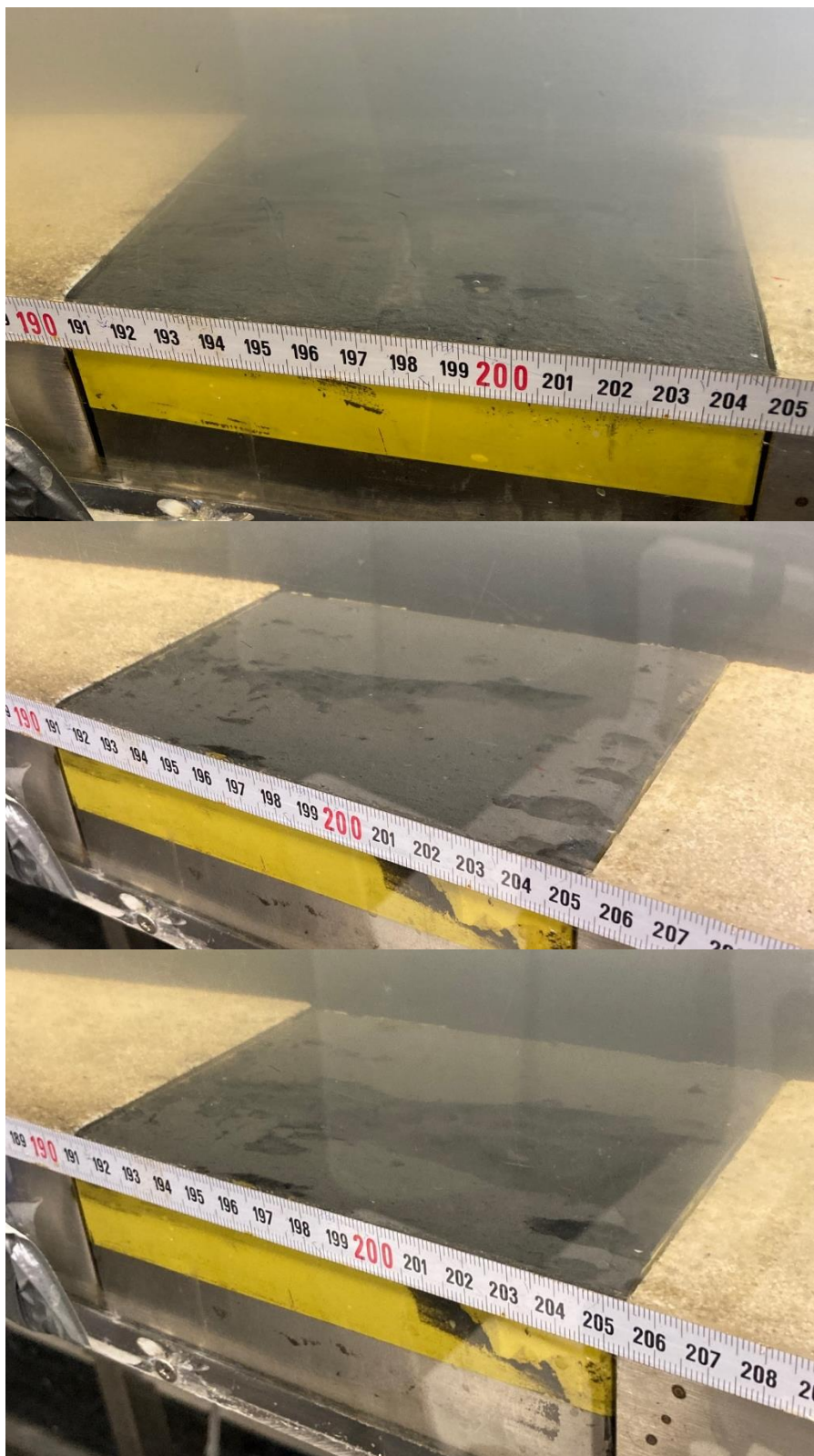
Figure 8-8: Pictures of flow-flume experiment PLUK1. Upper panel: at start of experiment, middle panel during experiment, lower panel: at end of experiment
