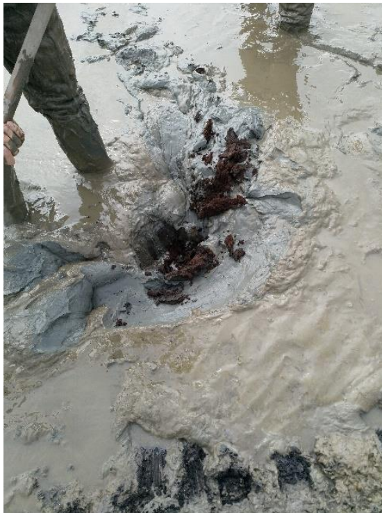
Figure 6-28: Pit made at location BATH3, where soft grey mud with a brown top layer overlays a peat layer, located at 0.20 m below the surface
