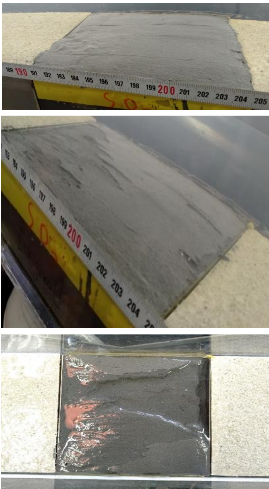
Figure 8-12: Pictures of flow-flume experiment SO3. Upper panel: at start of experiment, middle panel: during experiment, lower panel: at end of experiment
