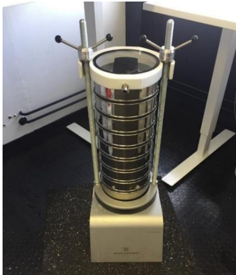
Figure 3-12: Haver & Boecker sieve stack
