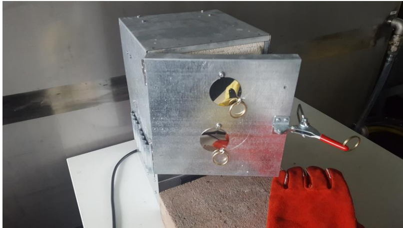
Figure 3-17: Furnace used to quantify the organic matter content through the LOI-method.
