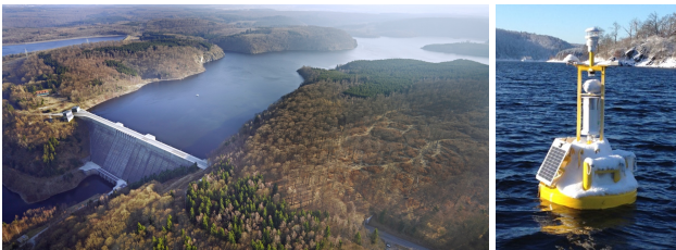
Figure 10: Left: Birds-eye view of the Rappbode reservoir, the site of the corresponding hydrological observatory. Right: Measurement buoy carrying sensors as employed in use case 2. Image source: UFZ.
