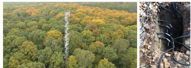
Figure 6: Left: Birds-eye view of the forest ecosystem observatory Hohes Holz. Right: Measurement set-up of multiple soil moisture sensors at different soil depths as employed in use case 1. Image source: UFZ.
