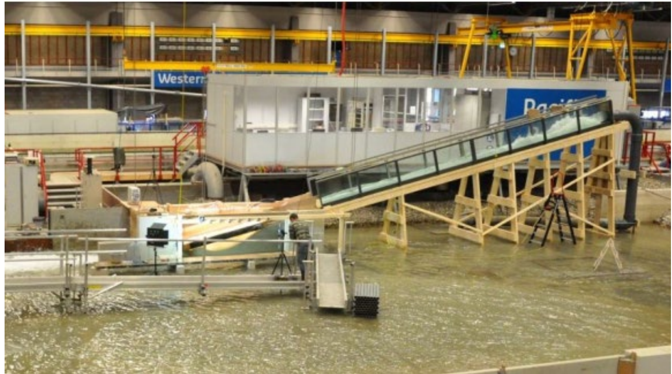
Previous indoor full scale test (erosion under crack in asphalt) at Deltares
