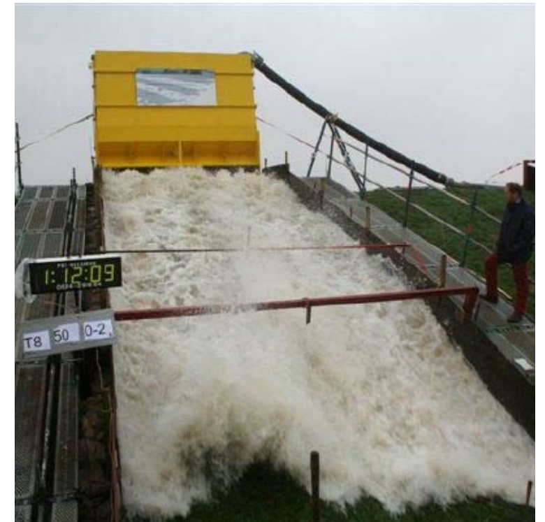
Overtopping flow inner slope, overtopping simulator
