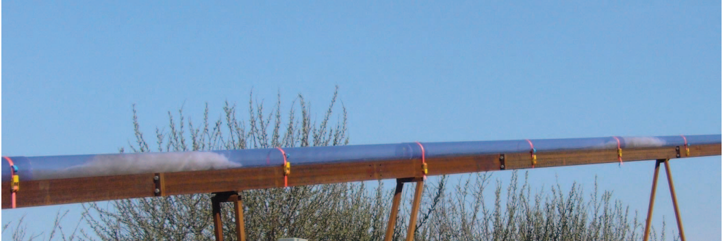
Figure 1: Subsequent hydraulic jumps in test rig (length 40 m, height 7 m) at wastewater treatment plant; water flows from right to left.
