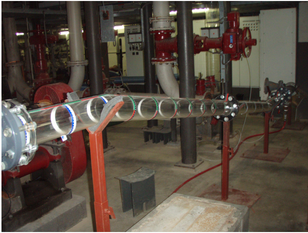
Figure 4. Layout of the 110 mm test section, \alpha = 10^\circ and L = 27D .
