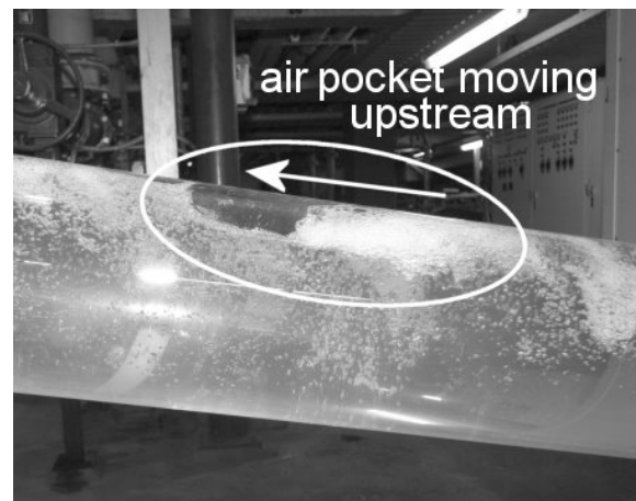
Figure 7: Dual mode flow, large slug moving upstream, small bubbles moving downstream.
