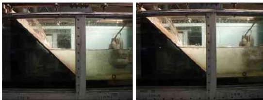
Waterhoogte is 40 cm Debiet is 10 l/s X is 1,5 m
