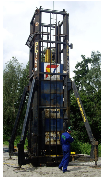
Rapid Load Testing load step 0.15 s (full test 2 hours) weight 7%
