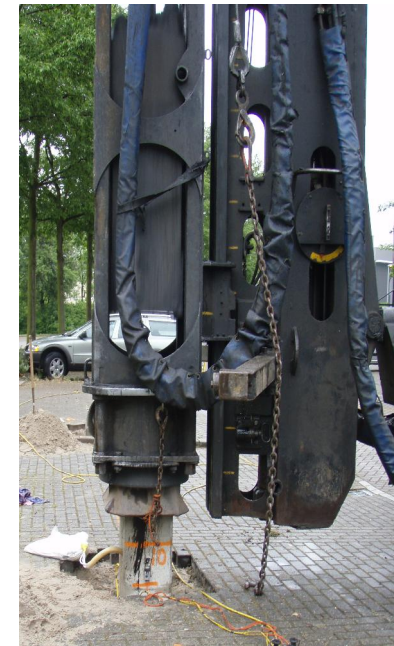
Dynamic Load testing load step 7 ms (full test 1 hour) weight 2%
