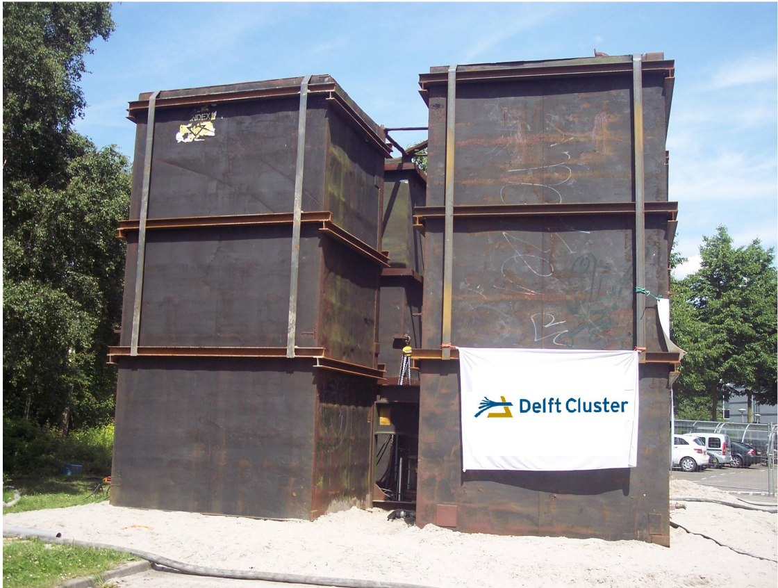
Photo 5.1 Water tanks used for static test
