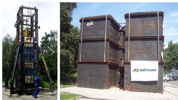
Figure 2 The Statnamic apparatus (RLT) and the counter weight (SLT)
