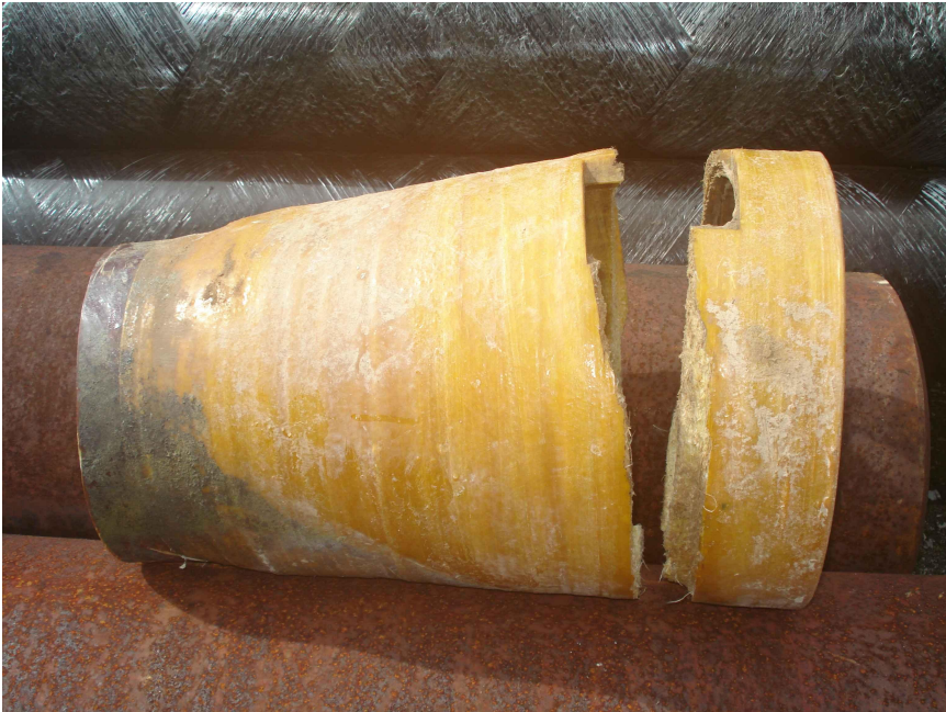
Figure 1: Damage to GRE-joint due to excessive axial loads.
