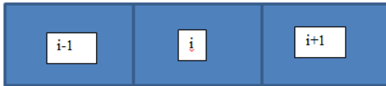
Figure 1, subdivision of pipe in elements for the temperature calculations
