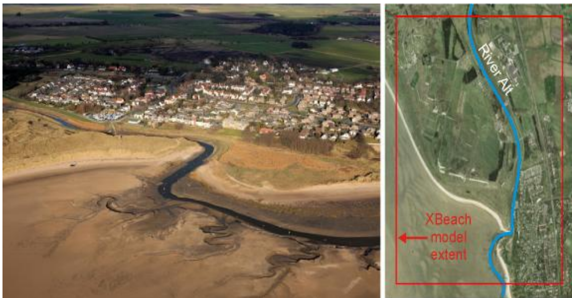
Figure 7.17 Oblique aerial photograph of the River Alt north of Hightown at low water (left panel); and GoogleEarth image of the River Alt showing the extent of the XBeach flooding model and the course of the river. Note the proximity of light industry and residential areas.
