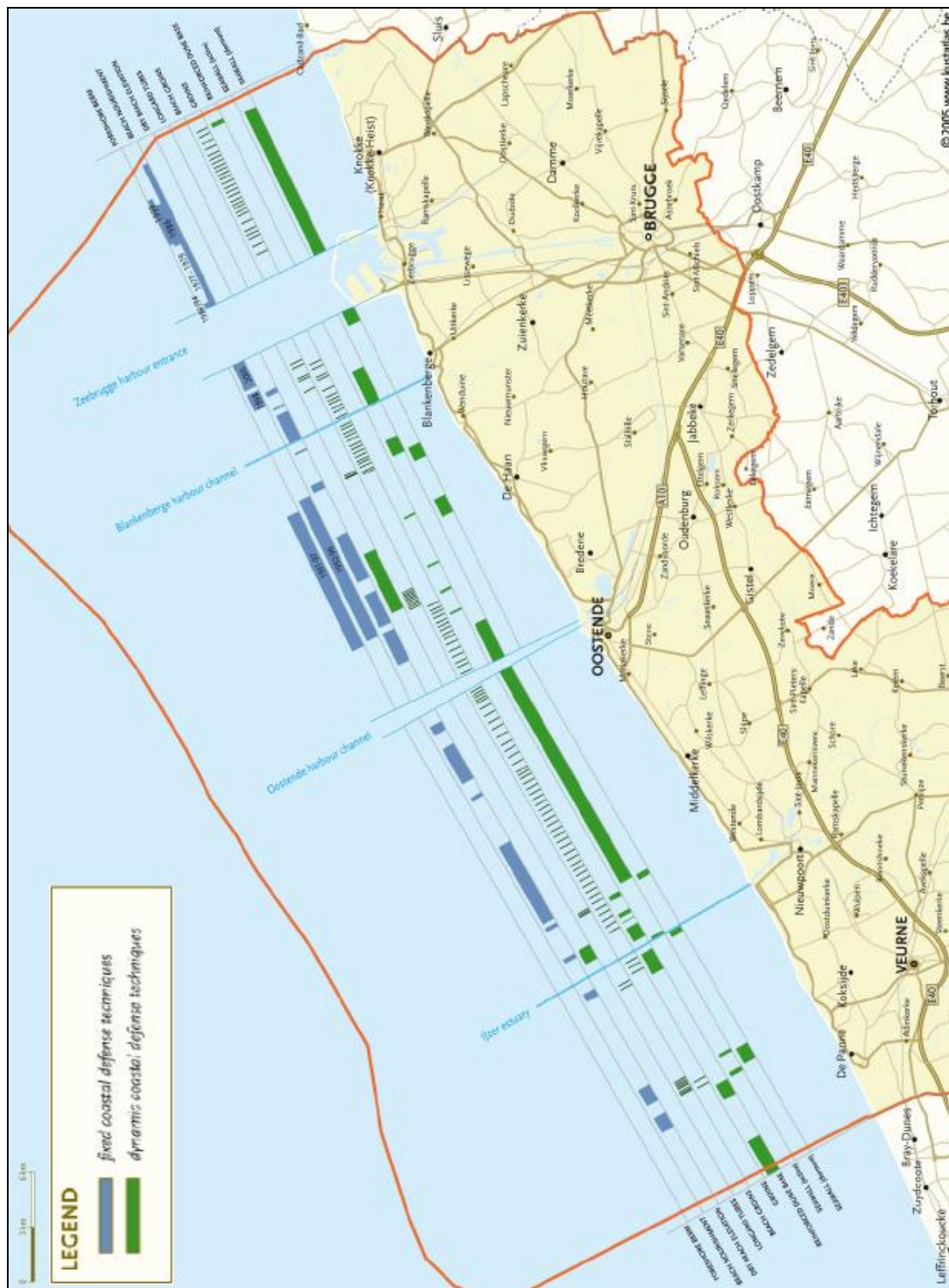
Figure 6.2 Overview of fixed and dynamic coastal defence techniques along the Belgian coast ( www.kustatlas.be ).
