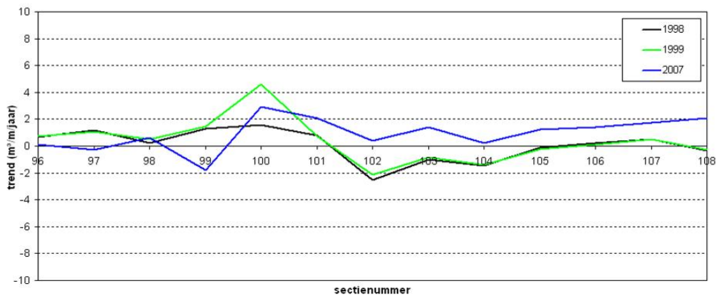
Figure 6.6 Comparison erosion/sedimentation trends wet and dry beach for 1998-1999-2007
