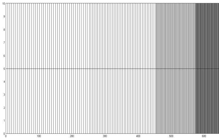
Figure 6.27 Figure 7 1: grid of the 1D XBeach model.
