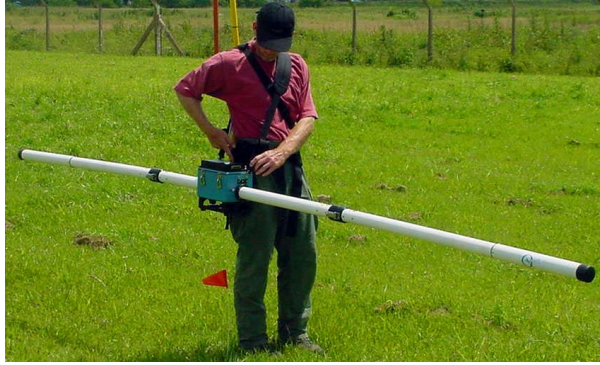
Figure 5: GEONICS EM31 as it is used in the field. Image credit: FPM Geophysical & UXO Services.
