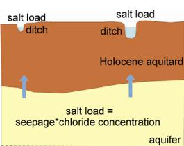
Fig. 6: concept of salt load to the surface water system.
