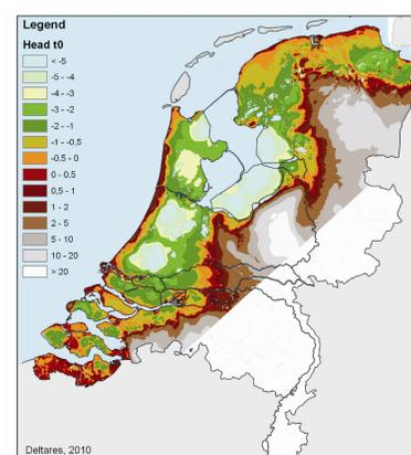
Fig. 8: Freshwater head [m] in the first aquifer.
