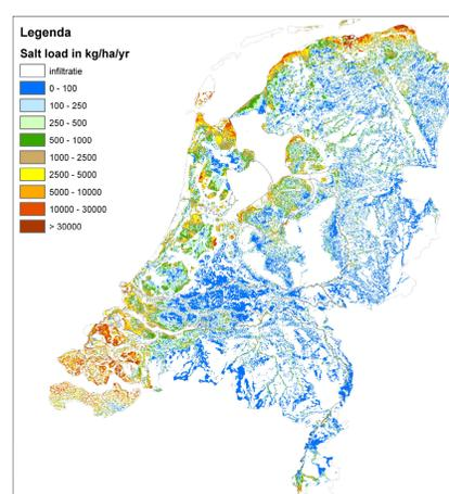
Fig. 7: Salt load to surface water system.
