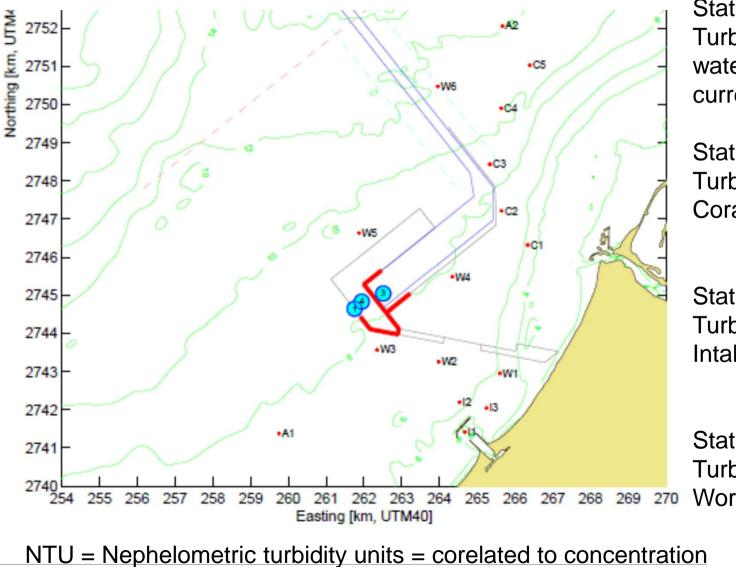
Stations A1-A2 Turb limit: [ - ] water levels, waves, currents, temp.
