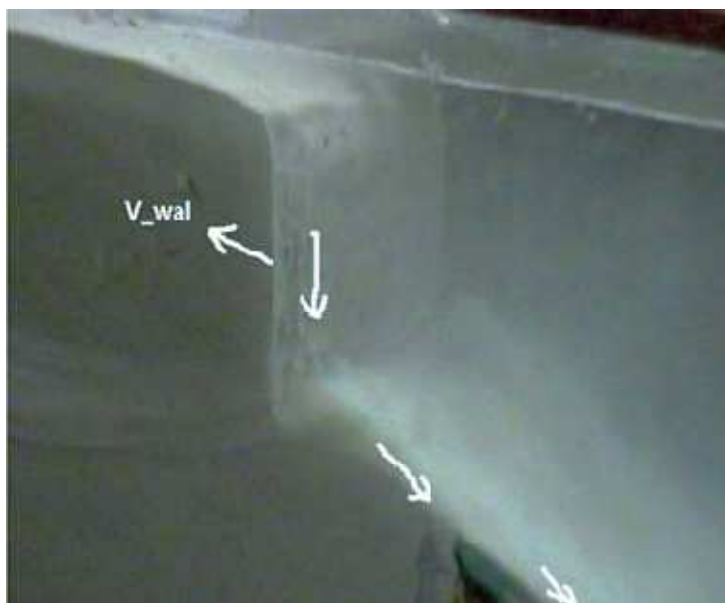
Figure 2.2-2: The process of a breach flow slide.
