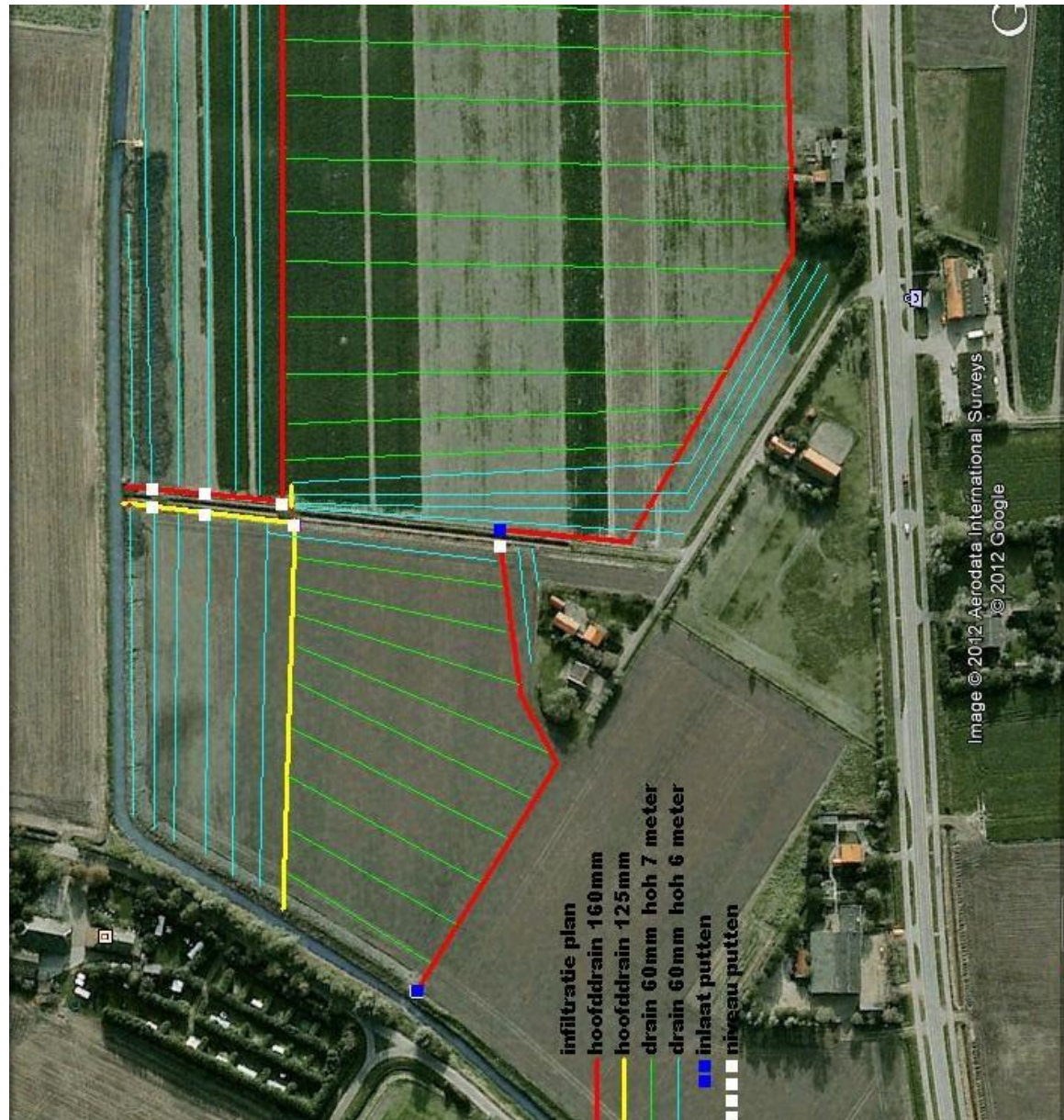
Figure I.2: Design of the pilot CCD system with infiltration facilities (Pauw and Van Baaren, 2012).
