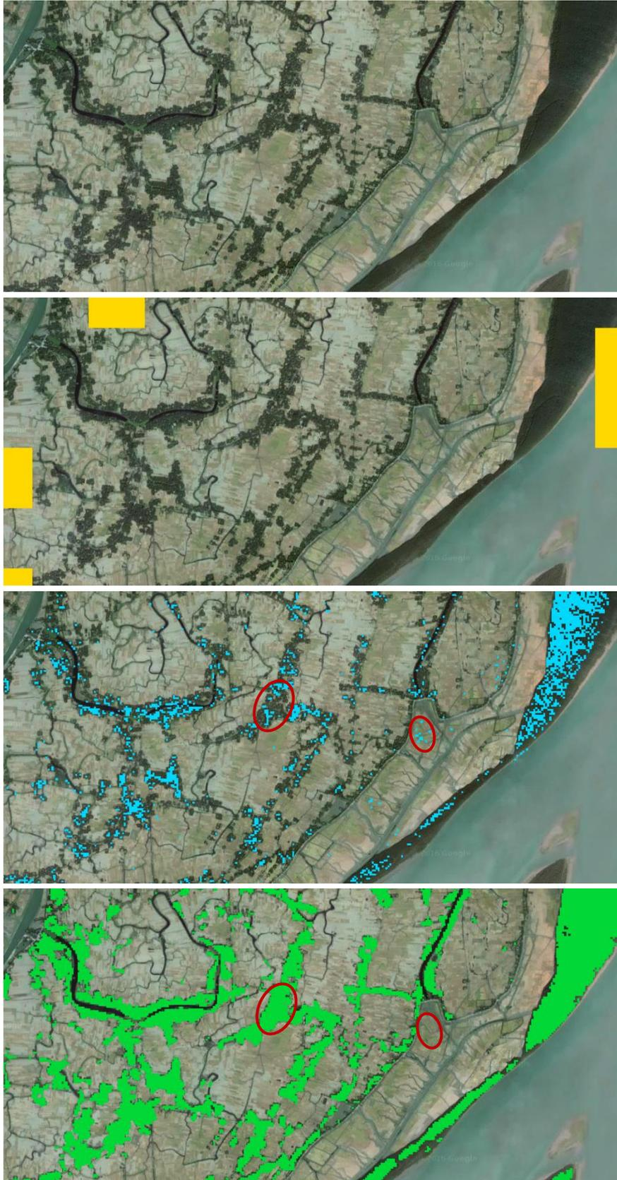
**Figure 15:** From top to bottom: 1) satellite imagery of a coastal polder (Rangabali) in the SC region; 2) Global forest canopy height map (Lefsky *et al.*, 2010); 3) Global tree cover map (Sexton *et al.*, 2013); 4) NDVI-based tree detection method, created in Google Earth Engine. The red circles indicate that the NDVI-based method (4) is able to differentiate between tree cover and high-productivity agricultural fields, while the Global tree cover map is not (3).
