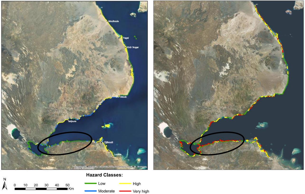
**Figure 30:** Manually classified (**left**) versus automated classified (**right**) gradual inundation hazard levels for the coastline of Djibouti
