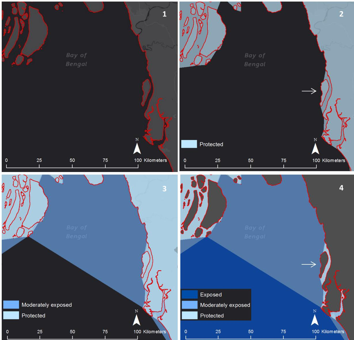
**Figure 16:** The intermediate steps of the automated free fetch estimation. 1) Original land features. 2) Land features within 10 km distance are connected. 3) Land features within 100 km distance are connected. 4) The final classification
