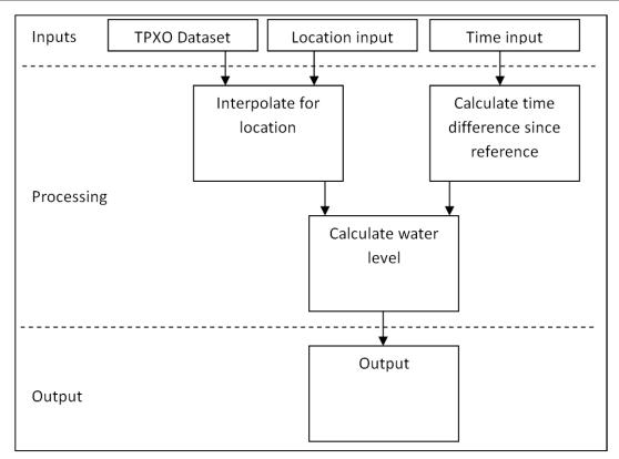
Figure 4.7 - Schematic view of the Tide Forecasting service.
