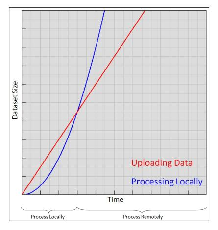
*Figure 2.8 - Use local or remote processing according to the uploading time of the dataset. (based on Michael and Ames, 2007)*
