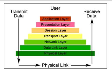
*Figure 2.11 - Schematized overview of the OSI model. HTTP is located in the Application Layer, CGI and SOAP are inside or on top of this. (Source: University of Washington, www.washinton.edu)*
