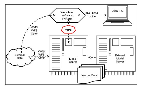
Figure 1.1 - Example of a WPS setup.
