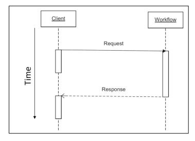
*Figure 2.9 - Example of an asynchronous request/response operation. After giving the request the client stops 'listening', when the process finishes a response is sent. (Zhao et al., 2012)*
