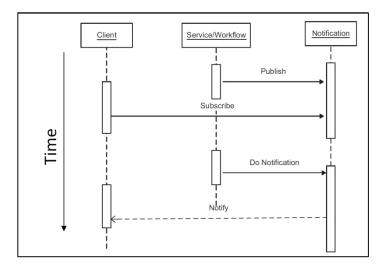
Figure 2.10 - An example of the Publish/Subscribe solution with the use of notifications. The client subscribes to the 'notification' on which the service publishes when the process is complete. (Zhao et al., 2012)
