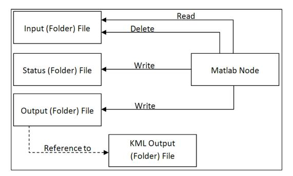
Figure 5.4 - Schematic view of the reading and writing cycle of the IDPT process.
