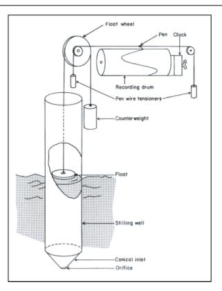
*Figure 4.2 - Schematic image of the working of a (classic) tide gauge with analogue recording. (Source: National Oceanography Centre UK, noc.ac.uk)*
