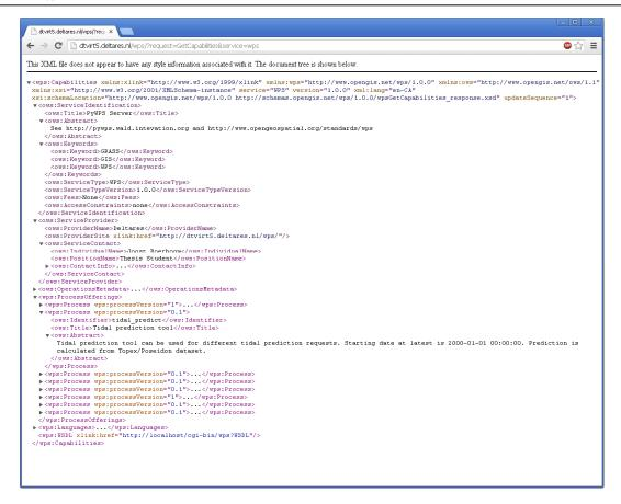
*Figure 2.2 - Example output of a GetCapabilities request. In the output document information can be found about for example the provider, available services and available languages.*
