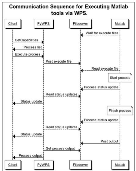
Figure 5.3 - Sequence diagram for executing Matlab tools using WPS via an external (model) server. The fileserver (FTP) is used as a bridge between the internet (client and PyWPS) and local network (Matlab).
