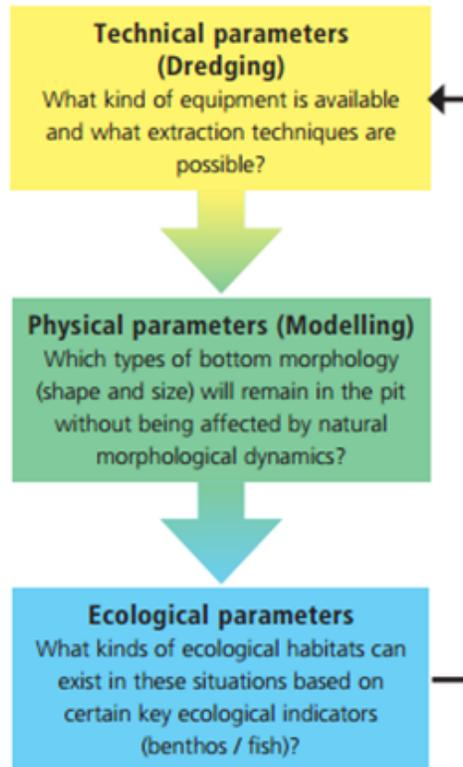
Flow chart showing the process used to accumulate requirements for designing the bed forms at existing extraction sites.
