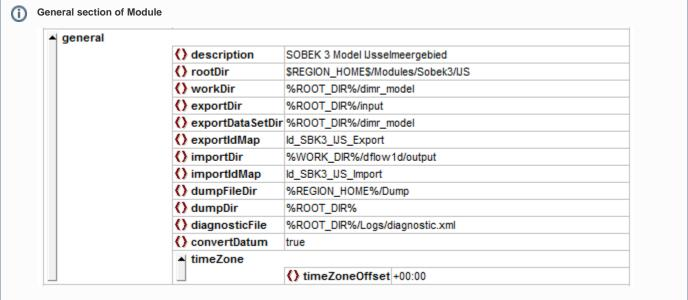
In the example configuration above it can be seen that the working directory of the DIMR should always be the folder ./dimr\_model. The Delft-FEWS exports timeseries to the folder .Vnput. After the modelrun is completed the output of the model is expected in the folder .\dflow1d/output.
