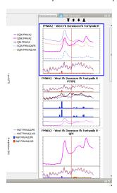
At the top of the panel there are four buttons. The first button selects the first plot, the second button selects the previous plot, the third button selects the next plot and the last button selects the last plot.
