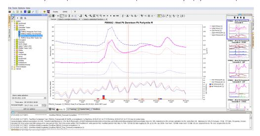
When the IFD is started, there is always at least one plot display available. This plot is called the primary plot display. The primary plot doesn't have lock icon at the left of the toolbar. When a new plot display is started this plot will have a lock icon at the left on the toolbar. When a new plot displayed is started, by default the plot will be locked. The lock icon is indicated in yellow in the image below.
