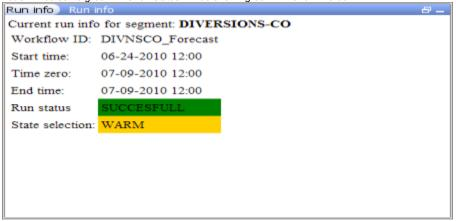
When the run is partly successful the icon of that node will be set to the red exclamation mark, the run status box in the run info panel will be set to yellow. When the run is failed the icon of the node will be set to the red exclamation mark, the run status box will be set to red.
