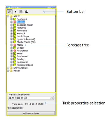
The forecast panel (indicated in yellow rectangle above) plays a central role in creating a forecast in the IFD. The forecast panel shows a tree with all the forecast points for a region and a logical grouping of these forecast points. It is also possible to show the work process of a forecaster in the forecast panel. The forecast panel consists of three main sections each of them will be explained in detail in the coming sections.
