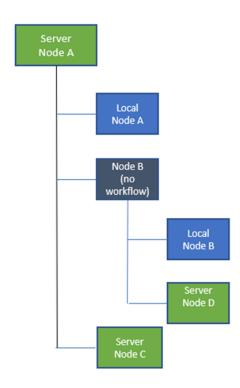
On the right is a schematic diagrams of a topology with nested nodes, which we will use to describe a different use case.
