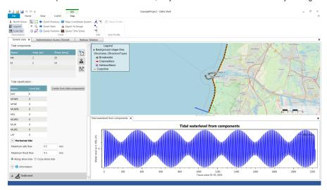
After the tidal components are available, the tidal signal can be classified in terms of Highest Astronomical Tide (HAT) up to Lowest Astronomical Tide (LAT). The definition can be found here. Click the Create from tidal components button to classify the tidal components.
