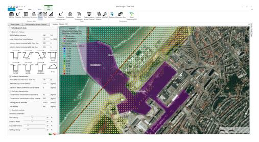
The horizontal eddy exchange volume depends strongly on the shape of the harbour entrance compared to the tidal flow direction/velocity. This factor needs to be given by the user (default = 0.03). The figure below helps to define this factor.
