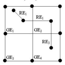
The groundwater model grid consists of four elements GE1, GE2, GE3 and GE4. These elements have the type Polygon. Each corner of these polygons is a Vertex, and each Vertex has Co-ordinates. The type Polygon is defined in the standard in the enumeration ElementType, whereas there are no interface definitions for Vertex and Co-ordinate; these are only part of the OpenMI terminology and are used in the naming of some of the methods in the IElementSet interface.
