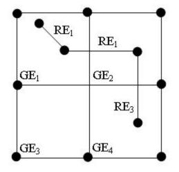
The groundwater model grid consists of four elements GE1, GE2, GE3 and GE4. These elements have the type Polygon. Each corner of these polygons is a Vertex, and each Vertex has Co-ordinates. The type Polygon is defined in the standard in the enumeration ElementType, whereas there are no interface definitions for Vertex and Co-ordinate; these are only part of the OpenMI terminology and are used in the naming of some of the methods in the IElementSet interface.
