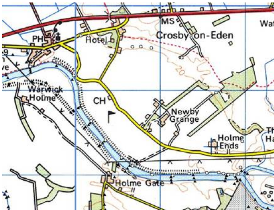
Figure 161 Example of a geo-referenced flood storage basin. Triangles indicate geo-referenced points. Empty circles (see the dotted selection line) show points belonging to a storage basin for which the 1D model provides one calculated water level.
