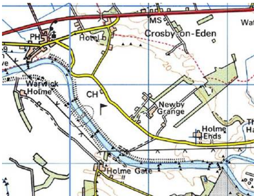
Figure 160 Example of geo-referenced cross sections. Triangles indicate geo-referenced points. Empty circles (see the dotted selection line) show points belonging to one cross section
