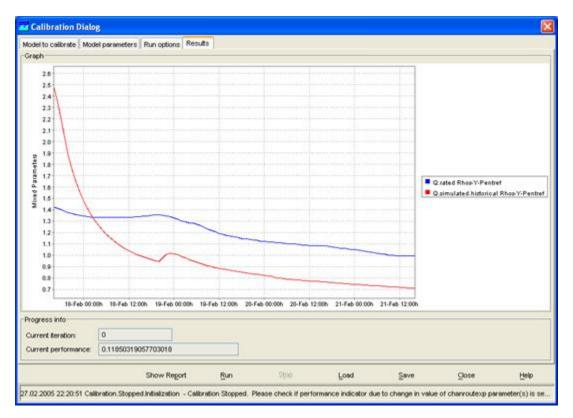
After the calibration run is completed you can select to see a report by pressing the [Report] button. The report of the calibration run contains information on the model parameters that have been optimised in each iteration step.
