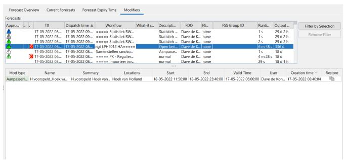
In the top panel the user can select the forecast workflow. Once selected the bottom panel will list all the modifiers that have been used. When the modifier is still active the first cell of the row is green, when it is inactive this cell is grey and the entire row is striked through.
